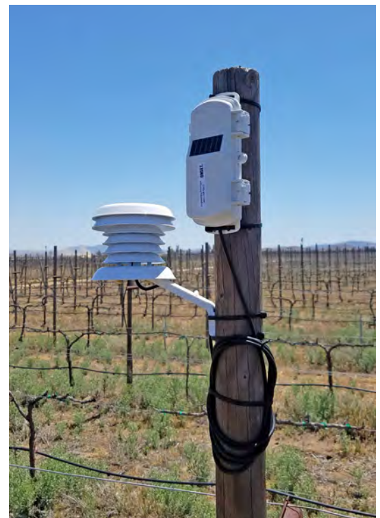
Look for wireless sensors that are small and that have integrated solar panels for easy deployment.
