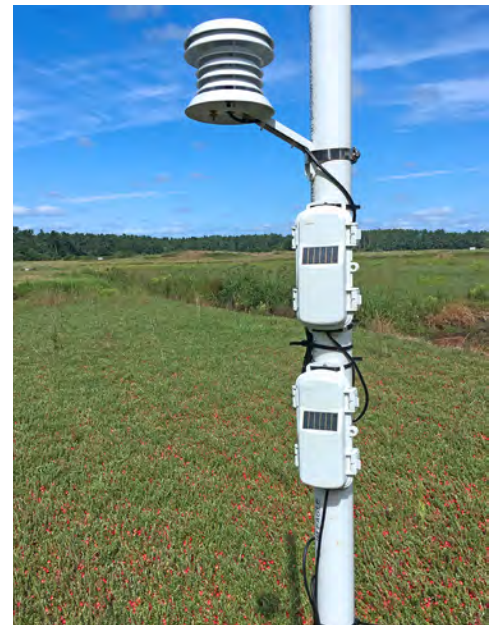
Monitor a wide area with a wireless field monitoring system.
