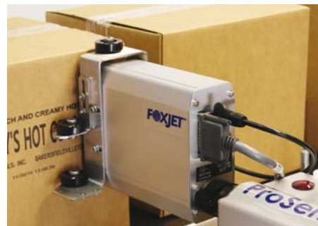
HIGH RESOLUTION PRINTING ON CASE
