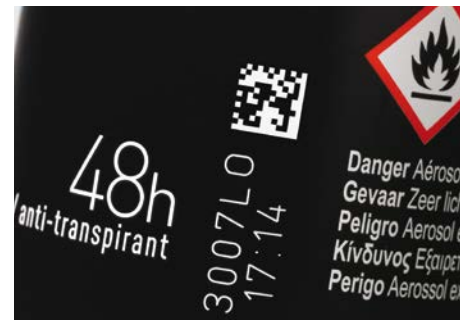
LASER MARKED 2D BARCODE
