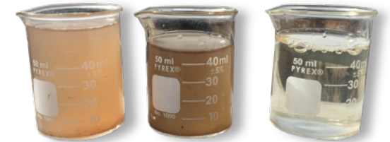
Headworks Post Primary Post BIDA®
