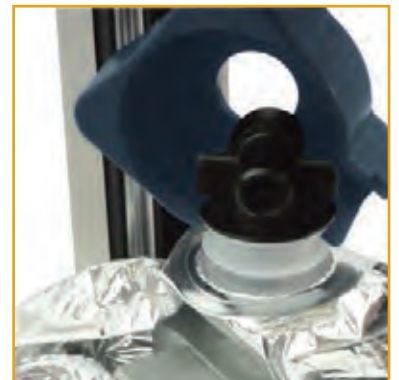
Tensile strength of sealed joint
