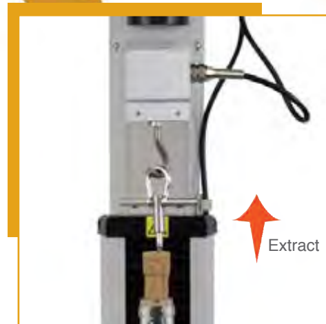
System converted to cork extraction tester
