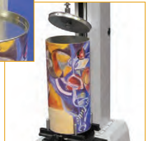
Lid removal test
