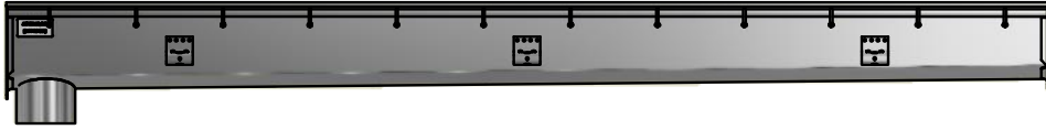
CHANNEL SECTION WITH BOTTOM OUTLET Standard NPS outlet sizes 1% slope and 0% (neutral slope) Toggle retaining tabs optional
