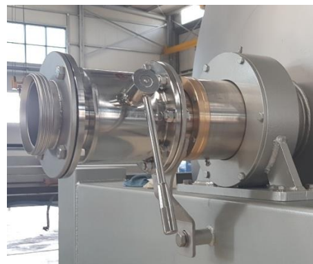
Stainless-steel loading ball valve, \varnothing 120 mm
