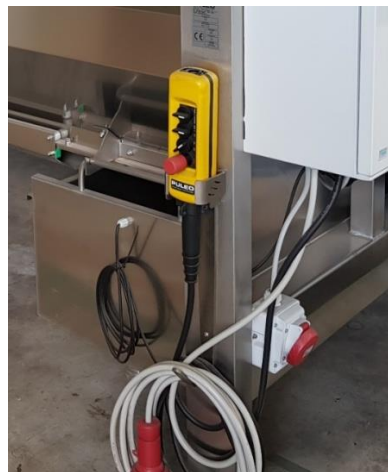
Electromechanical manual commands on a pushbutton control board with cable
