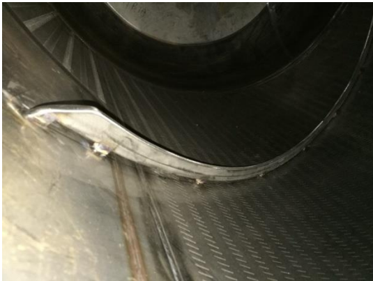
Stainless-steel conveyors for marcs discharge
