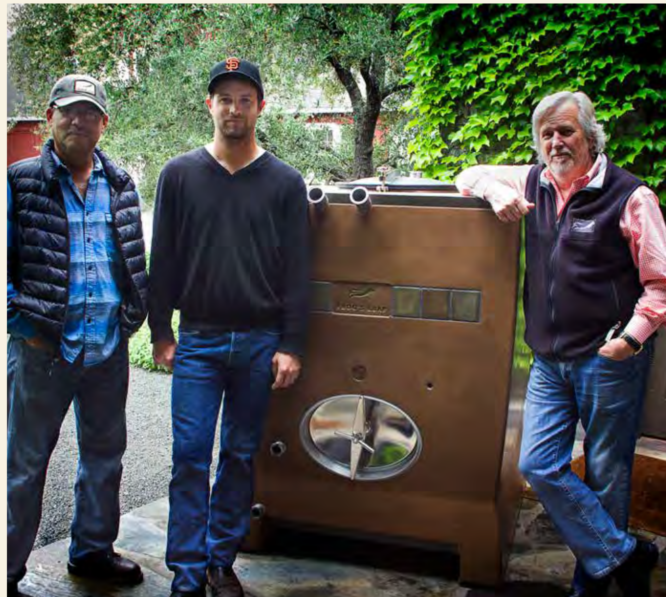
Current design has pomace door set lower than shown here to facilitate cleaning.
