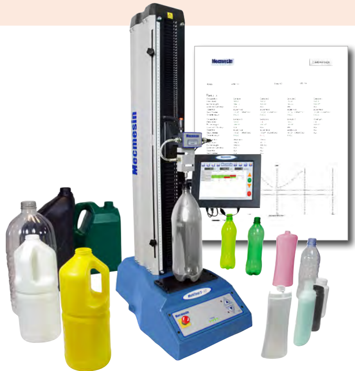
Top-load test on PET bottle using a MultiTest 5-xt Touch Screen Controlled Tester. Generate your own report with full test data
