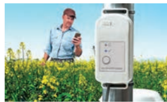
On-site monitoring (Using Bluetooth BLE and HOBOMobile)
