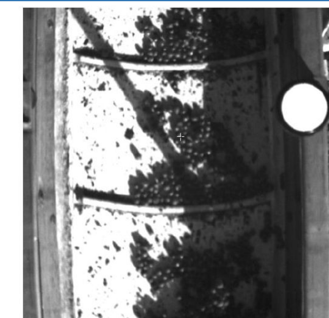
Figure 4. Example of hyperspectral imagery from the harvester conveyor (here at 640nm). The white circle on the right is a reflectance standard.
