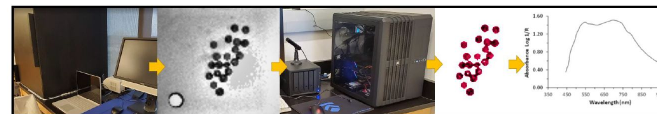
Figure 1. Hyperspectral imaging of berry samples in the lab. Hyperspectral images are acquired in a dark cabinet with a consistent light source. Berries are imaged together with a reflectance standard (here image is taken at 520nm). The datacube (Height x Width x Wavelength) is processed in a powerful workstation, pure berry pixels are extracted from the picture, and it is possible to obtain an average absorbance spectrum (here VIS/NIR), but also individual spectrum for each berry (and each pixel in a berry). These data can be used for modeling purposes.
