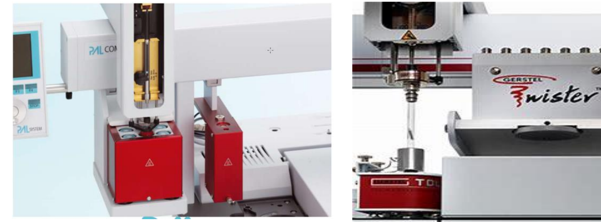
Fig 3. Headspace-GC-FID and SPME-GC-MS for major volatile analysis (left), SBSE-GC-MS for C 13 -norisoprenoids (right).
