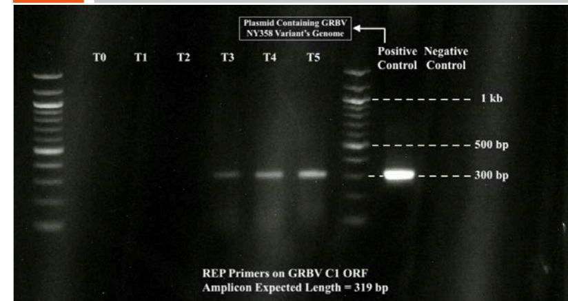
Figure 4 - 1.5% Agarose gel run. Total RNA has been extracted at each sampling date and used as template for reverse-transcription PCR (RT-PCR). The expected amplicon length was 319 bp. A plasmid containing the GRBV genome (variant NY358) has been used as positive control in the RT-PCR reaction, while the negative control is represented by water. The plasmid containing the GRBV genome has been provided by Keith Lloyd Perry (Cornell University).
