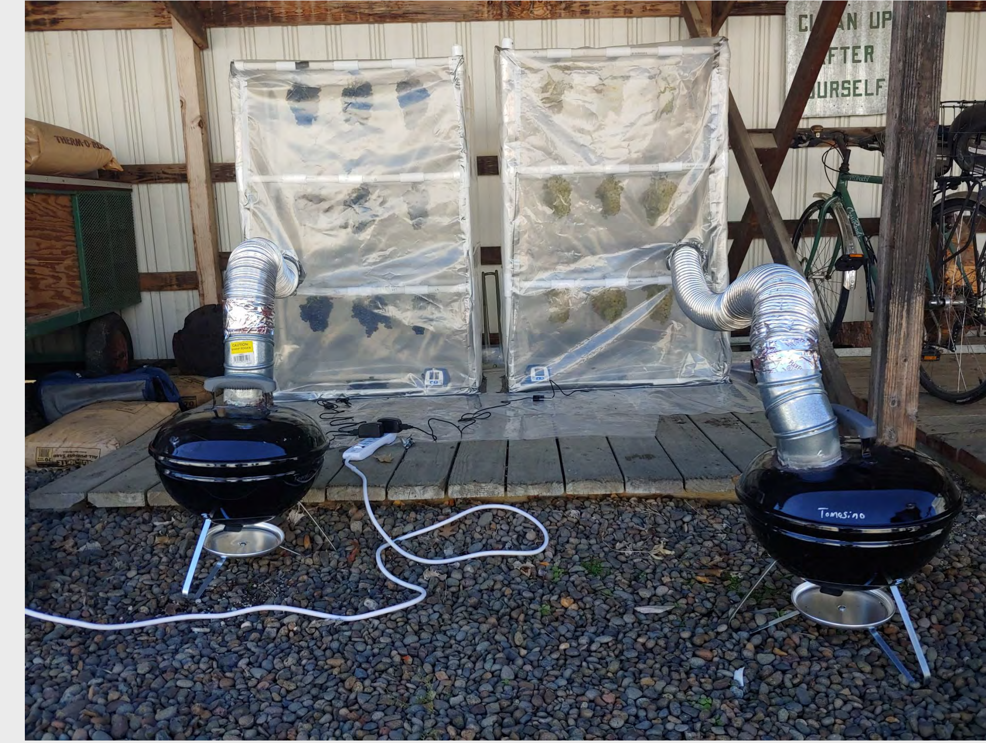
Figure 4 – 5 g barley burned and piped “cold” for smoke transfer to pinot noir (left) and chardonnay (right) wine grapes, 1\ \mu\text{m} smoke particle density maintained > 70\text{ mg/m}^3
